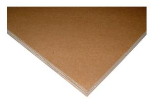
**Primer:** Use a good primer. Prime both sides of the MDO board and all the edges of the sign board with at least two coats. Grey may be a better choice for the primer color or white.
