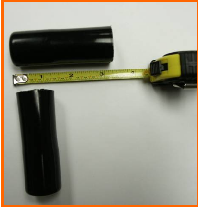
Figure 1. Rumen temperature bolus measures approximately 3.25 inches long and 1.25 inches in diameter.
